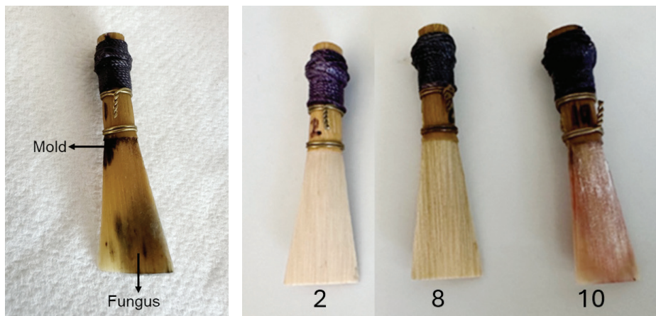
Figure 1 (left). Reed 1 (water rinsed and shake dry) on day 13 showing aggressive mold and fungus growth.
